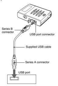
If a plug is already connected to the USB port connector of your PC, disconnect it before connecting this player.
